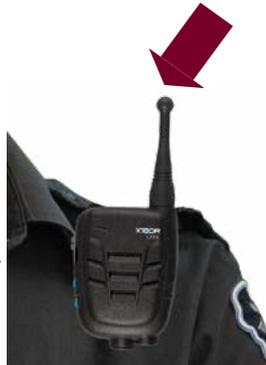
**Gateway Off/On:** press for 1 second, gateway and Blue LED turns on. Press again for 1 second and gateway and Blue LED turn off.
